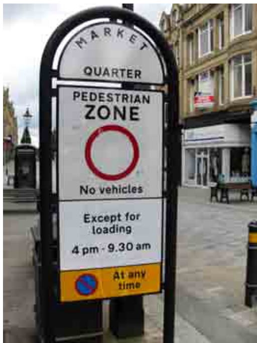
Groups of signs should be coordinated or combined into one panel to avoid clutter
