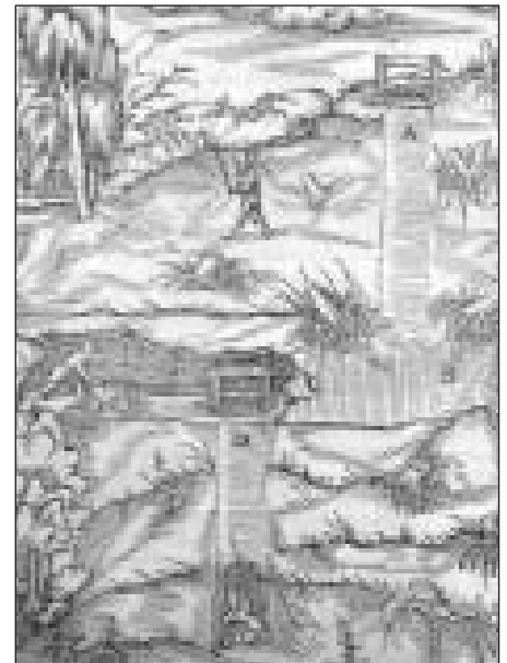
A cross section of the workings showing multi level winding in place.
