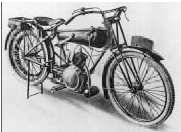
The racey lines of the H.C.L. motorcycle, showing Villiers engine, hand gearchange and belt drive to rear wheel.
