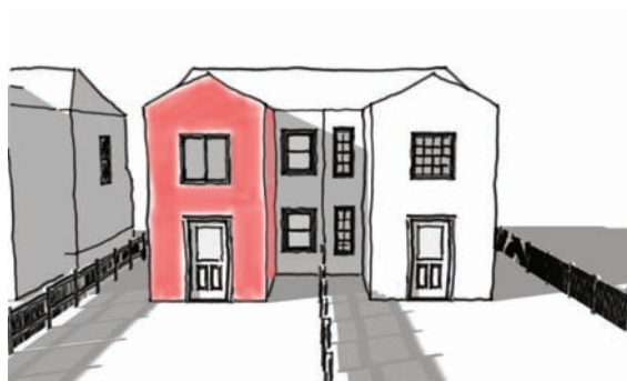
Creating the 'tunnel effect' can affect a neighbours residential amenity
